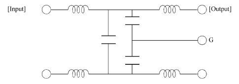
Figure 4.8 AC noise filter (recommended)
